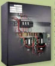
Lutron installs continuous duty thermal magnetic breakers in all of its dimming panels. A typical magneticonly breaker has a magnetic element that senses large fault currents that cause it to trip. A thermal magnetic breaker has both a magnetic and a thermal element. The thermal element senses small overloads which heat
